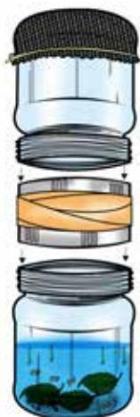
Assemble the nursery by screwing together two bottles that we provide. The bottle built with the mesh screen goes on top, to allow the mosquitoes to breathe during their aquatic and adult stages. The screen also prevents adult mosquitoes from escaping from the nursery.
